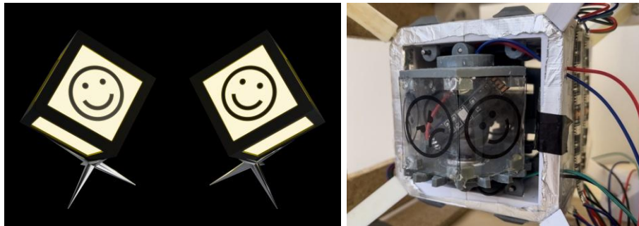
Figure 2. 3D rendering of a model showing how we envisioned Emoji Lantern during the design process and the shadow projector of our final prototype.
